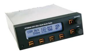
Combined 8.33 kHz Voice COM and VDL Mode 4 transceiver, RTX6040
